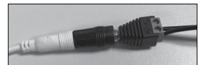
Wires connecting to power port on Simplicity shade: supplied.
